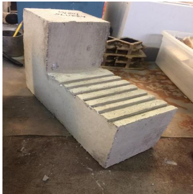
Figure 3: L-shaped underlay half after 18 hours of steam curing
